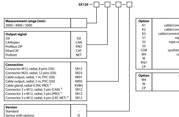
Description cable/connector orientation top cable/connector orientation left cable/connector orientation bottom rope outlet sideways top rope outlet sideways bottom rope outlet bottom synthetic wire rope (Coramid) rope fixation M4 thread rope fixation eyelet protection class IP67 corrosion protection not combinable with СР P
