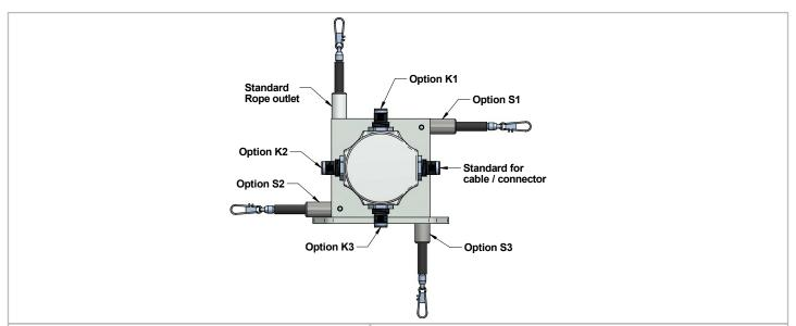
The sensor is usually installed by using the regular mounting plate | Sensors with option rope outlet S2 and S3 have a modified base plate: (see technical drawing above).
